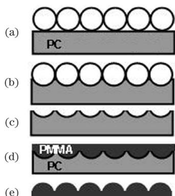
Fig. 1. Schematic of the fabricating processes. (a) Self-assembly of silica microspheres on the surface of the PC substrate; (b) embedding of silica colloidal crystal under heat treatment; (c) forming of PC microcavity arrays after dissolving the silica microspheres by a HF solution; (d) a pattern transfer achieved by using hot embossing technique; (e) a HCP replica of hemispherical PMMA convex MLAs obtained after peeling off the PC mold.
