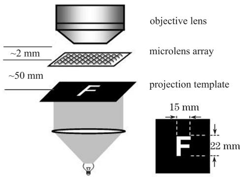
Fig. 3. Schematic of the projection experiment. The projection object is a transparent letter ‘F’ with a size of 15×22 (mm).
