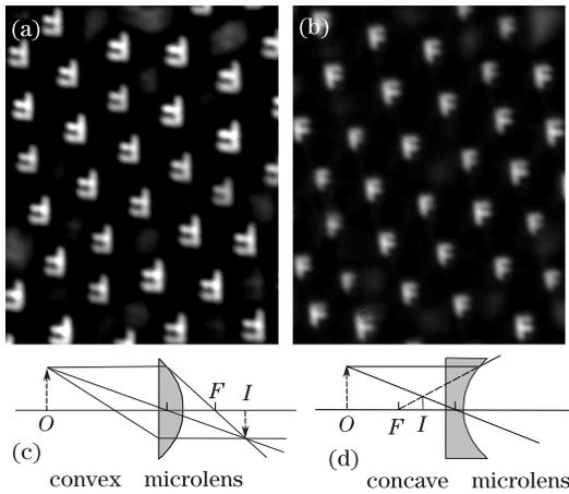
Fig. 4. Comparison of the optical micrographs of the images projected through (a) PMMA convex microlenses and (b) PC concave microlenses. (c), (d) Beam paths for (c) the convex lens and (d) the concave lens, respectively.
