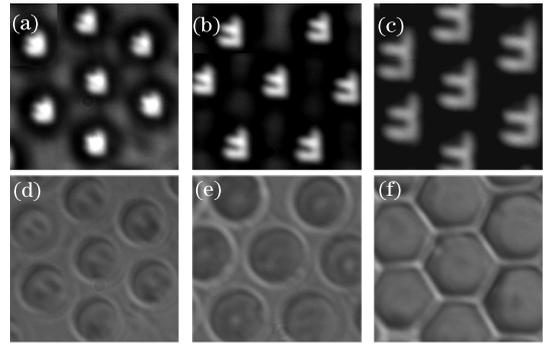
Fig. 5. Comparison of the inverted letters ‘F’ projected through the convex microlenses with diameters of (a) 3.25, (b) 4.12, and (c) 5.0 μm, respectively. (d)–(f) Optical micrographs of three microlenses corresponding to (a)–(c) where the unclear edges are due to the optical diffractions.
