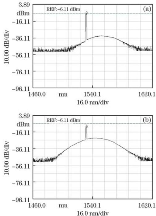
Fig. 4. Reflective spectra of the RSOA with input power of (a)  $-1.70$  dBm and (b)  $-21.11$  dBm.
