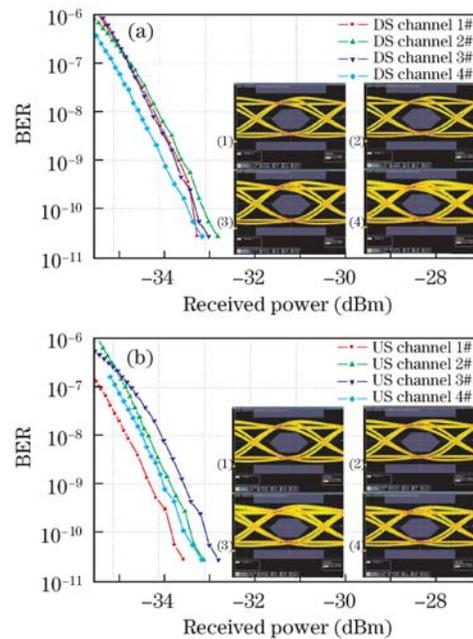
Fig. 2. BER versus received power for (a) DS and (b) US of the four channels. Insets: eye diagrams of (1) channel 1 after 20-km transmission, (2) channel 2 after 40-km transmission, (3) channel 3 after 60-km transmission, (4) channel 4 after 80-km transmission.
