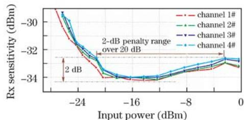
Fig. 5. Rx sensitivity of US signals for four channels.
