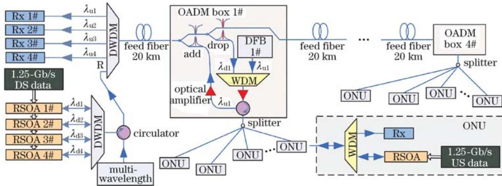
Fig. 1. Architecture of distributed access LR-HPON with OADMs. Rx: receiver; DWDM: dense wavelength division multiplexer; ONU: optical network unit.
