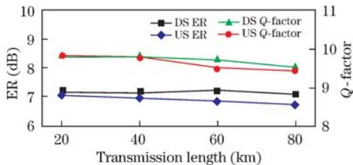
Fig. 3. ER and  $Q$ -factor versus transmission length at BER of  $10^{-10}$ .
