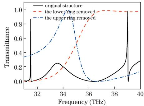
Fig. 4. (Colour online) Transmittance as a function of frequency for three cases. The solid black curve (i.e., the curve in Fig. 2) represents the original structure. The dashed red curve shows the case when the lower ring is removed. The dash-dot blue curve shows the case when the upper ring is removed. The other parameters are the same as those in Fig. 2.
