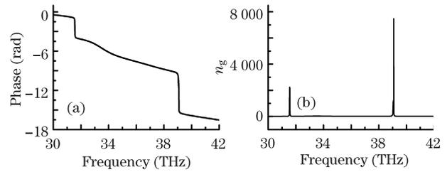
Fig. 3. (a) Transmission phase and (b) group index as a function of frequency.
