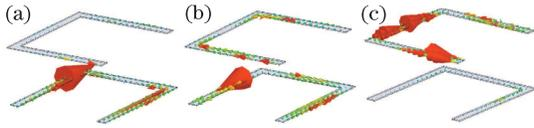
Fig. 5. (Color online) Current distributions in the two rings at resonance frequencies of (a) 31.56 (the first resonance), (b) 33.62 (the second resonance), and (c) 39.04 THz (the third resonance) in Fig. 2, respectively.
