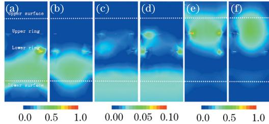
Fig. 6. (Color online) Electric field distributions in different cross-sections at different resonance frequencies in the unit cell. Electric field distributions at (a) section 1 and (b) section 2 corresponding to Fig. 1 at 31.56 THz; electric field distributions at (c) section 1 and (d) section 2 corresponding to Fig. 1 at 33.62 THz; electric field distributions at (e) section 1 and (f) section 2 corresponding to Fig. 1 at 39.04 THz.
