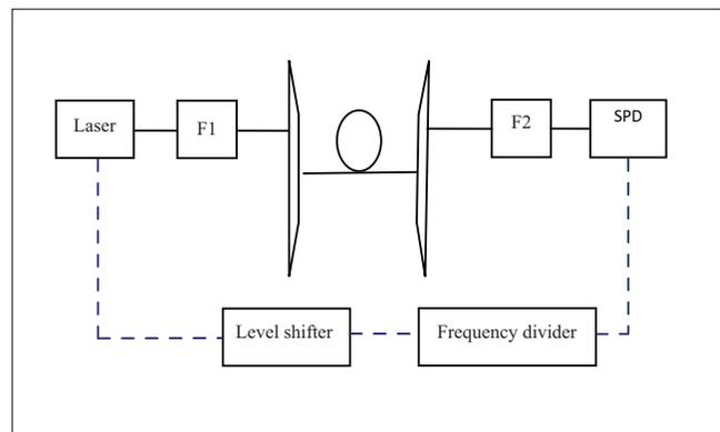
Fig. 1. Stokes Raman scattering noise test setup. Solid lines indicate the route of optical signal and dotted lines indicate the route of electrical signal. F1, 1310-nm filter; F2, 1550-nm filter.
