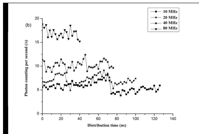
Fig. 3. Experimental data of photon counting of anti-Stokes Raman scattering noise when the SMF length is (a) 25 and (b) 50 km.
