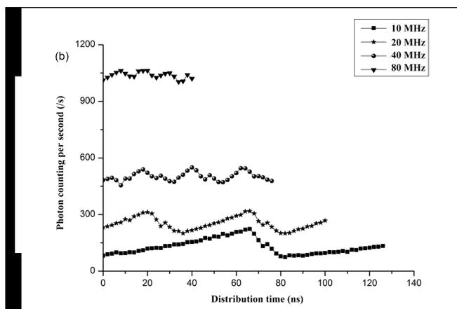
Fig. 2. Experimental data of photon counting of Stokes Raman scattering noise when the SMF length is (a) 25 and (b) 50 km.
