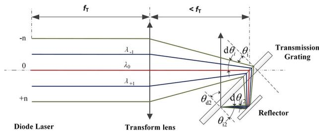
Fig. 2. Schematic of the proposed approach with a double-pass transmission grating and reflector.
