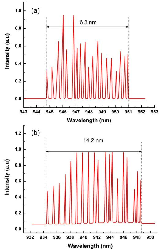
Fig. 3. (a) Spectral characteristic of the system with a single grating and double pass using a reflector. (b) Spectral characteristic of a conventional SBC laser.
