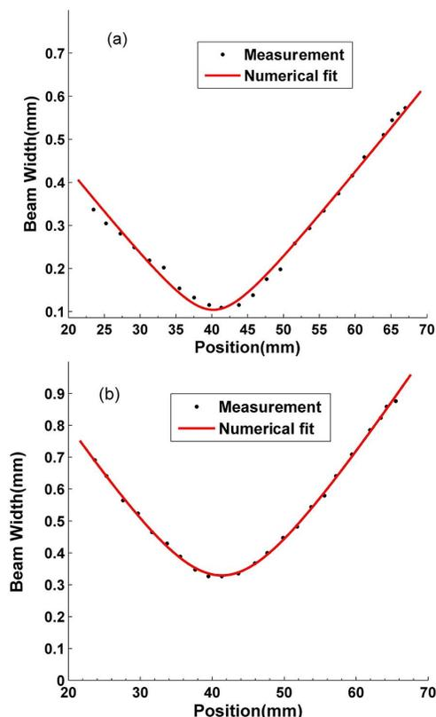
Fig. 5. Beam quality measurement of the diode laser array after SBC using numerical fits. (a) Fast axis. (b) Slow axis.
