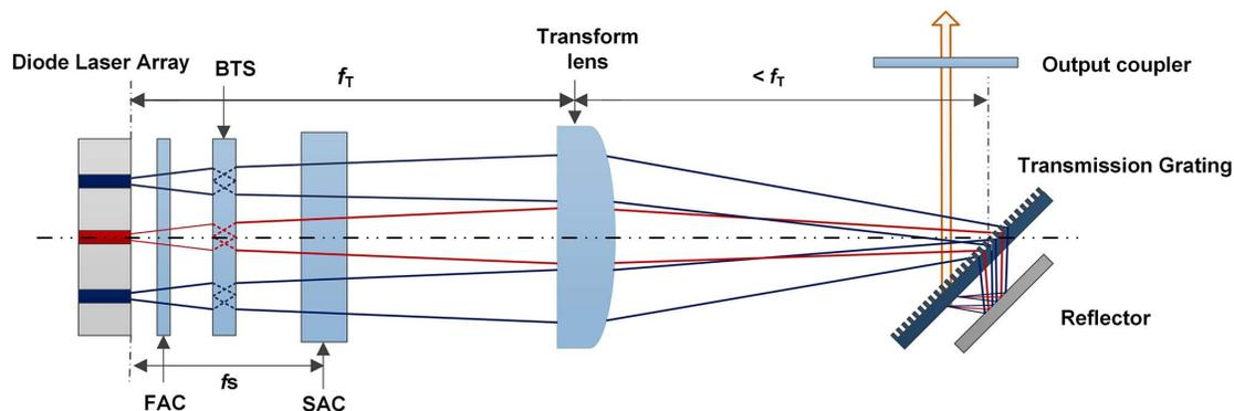
Fig. 1. Schematic of the SBC system with a double-pass transmission grating and reflector.
