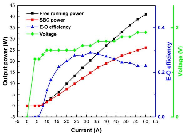
Fig. 4. CW output power and E-O efficiency.
