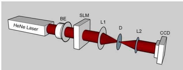
Fig. 5. Experimental setup. From left to right: He–Ne laser at 633 nm, 12 mW; BE, beam expander, 10 $\times$ ; SLM, spatial light modulator, LC2002; L1 and L2, lenses; D, diaphragm; CCD, Thorlabs CCD.
