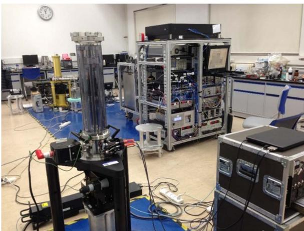
Fig. 7. Atom gravimeter runs normally in the test site. The test sites are well-isolated from vibration, and the temperature and humidity in the test room are well controlled.
